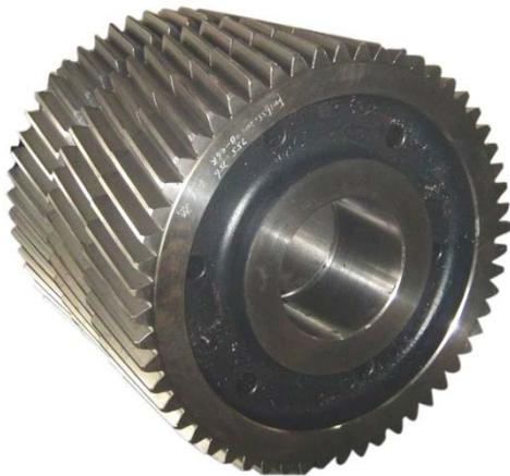
The leading edges of the teeth are not parallel to the axis of rotation, but are set at an angle. Since the gear is curved, this angling causes the tooth shape to be a segment of a helix. Helical gears can be meshed in parallel or crossed orientations. The former refers to when the shafts are parallel to each other; this is the most common orientation. In the latter, the shafts are non-parallel, and in this configuration the gears are sometimes known as "skew gears".
