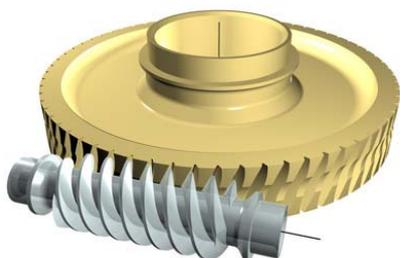
A gearbox designed with a worm and worm-wheel will be considerably smaller than one made from plain spur gears and has its drive axes at  $90^\circ$  to each other. Given a single start worm, a 20 tooth worm gear will reduce the speed by the ratio of 20:1. With spur gears, a gear of 12 teeth (the smallest size permissible, if designed to good engineering practices) would have to be matched with a 240 tooth gear to achieve the same ratio of 20:1.
