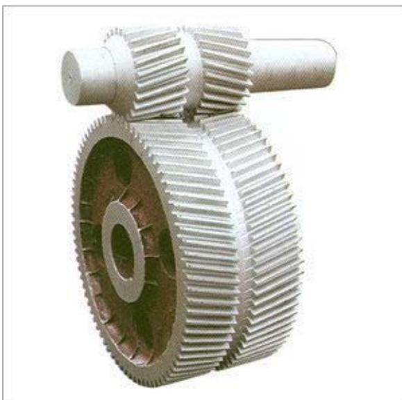
The teeth of these wheels are made in the form of the letter «V». Programs based on such gears, commonly called "herringbone". Chevron wheel solves the problem of the axial force. Axial forces of both halves of the wheel cancel out, so there is no need to install the shafts on ball thrust bearings.
